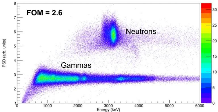
nEL crystals incorporate 7% 6-Li permitting thermal neutron detection, while Cl-35 enables fast neutron detection. The emission of nEL is comprised of fast core-valence luminescence (CVL) and Ce related emission resulting in two main decay components. Absence of CVL under neutron excitation allows for easy discrimination between the neutron and gamma radiation. An FOM value of 2.6 was achieved using a Pu/Be neutron source.
