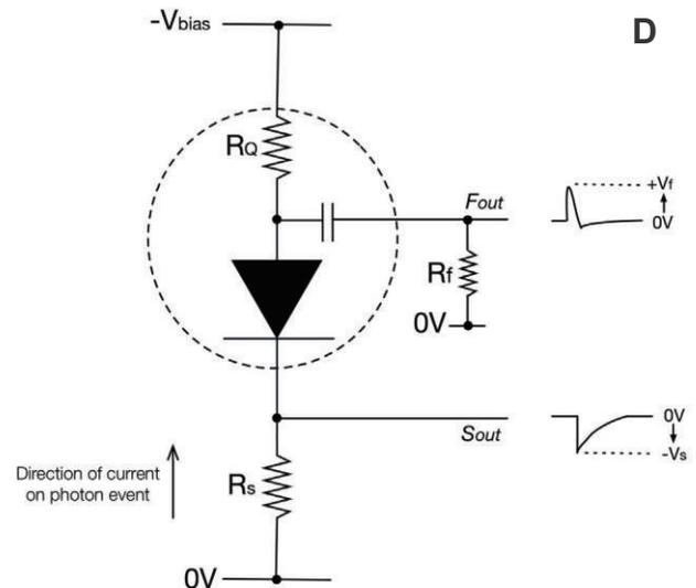
Ref.: J-Series High PDE and Timing Resolution, TSV Package, Datasheet, SensL
