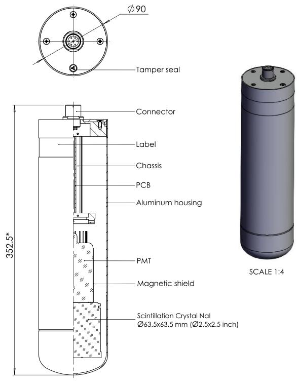
\* The length of Scintillation Probe may vary depending on connector type
